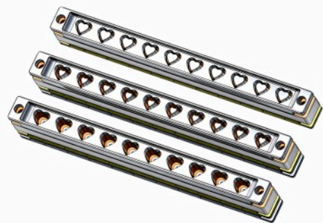
双色口红模具 Dual-color lipstick mold
